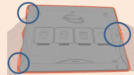
Verify that the iPad is securely held by the hooks to the left and the locking clip to the right.
