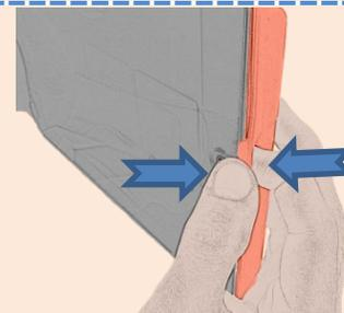
Gently push the locking clip outwards with your thumb while simultaneously pushing the iPad out of the enclosure with your index finger.
