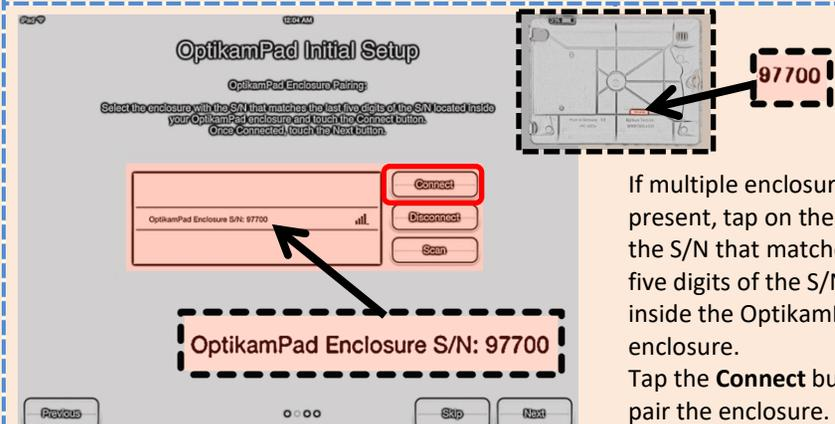
If multiple enclosures are present, tap on the one with the S/N that matches the five digits of the S/N located inside the OptikaMPad enclosure. Tap the **Connect** button to pair the enclosure.
