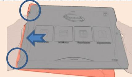
Ensure that the iPad slides under the hooks located to the left of the enclosure.
